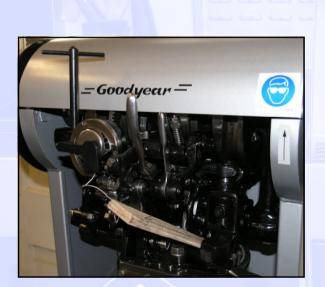
Standard Goodyear Head with T Bar shuttle case lock
