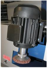
Naumkeag Guard on shaft (a protective sleeve prevents accidental gripping of the naumkeag shaft)
