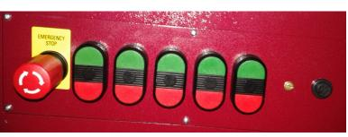
The Emergency Stop will stop all electronically controlled equipment on the finisher. To reset, the red knob must be twisted and released.
